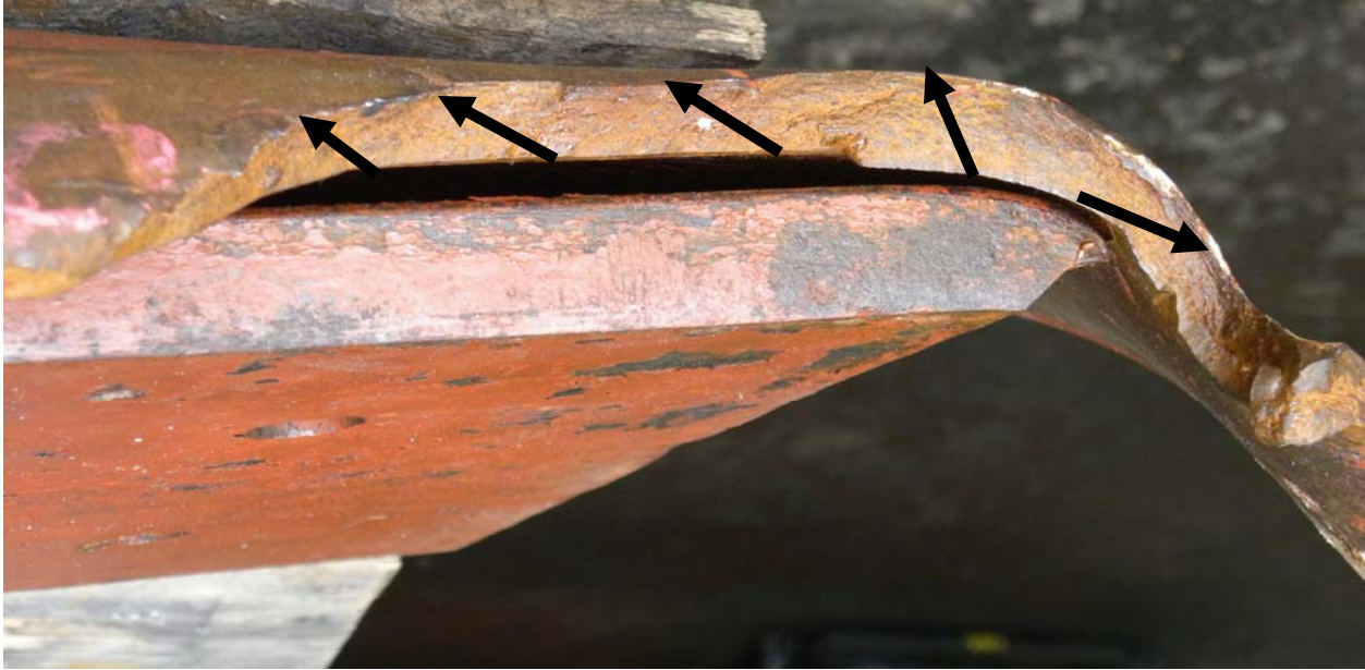
Figure 5: Close-up view of Fracture 1 on base side of fracture. Arrows show directions of fracture propagation. Morphology is consistent with fracture morphology after severe buckling has occurred.
