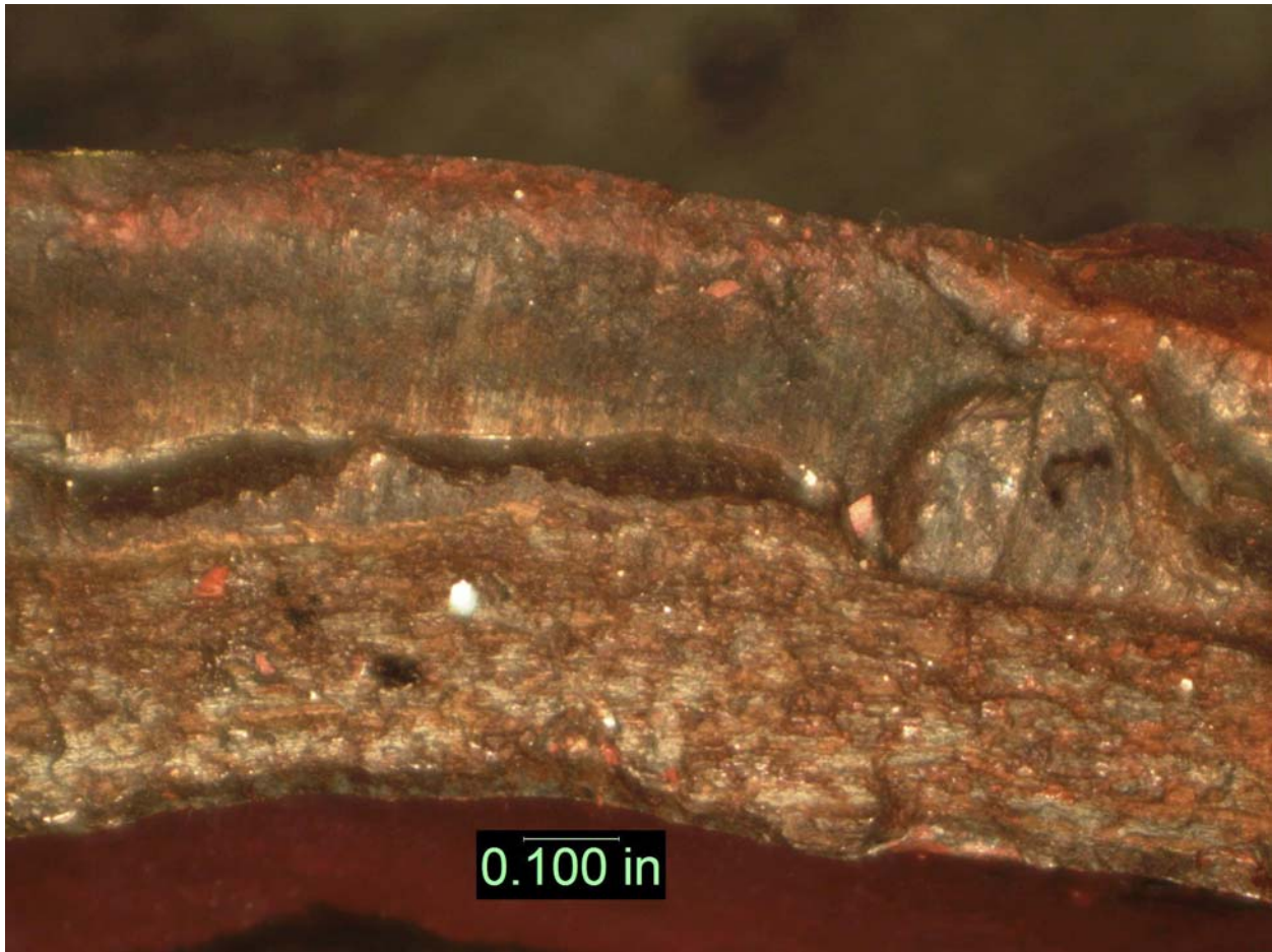
Figure 10: Macroscopic view of area outlined in Figure 9 shows a lack of fusion above the ridge line, as indicated by parallel machining marks which were on the edge of the original member being welded.
